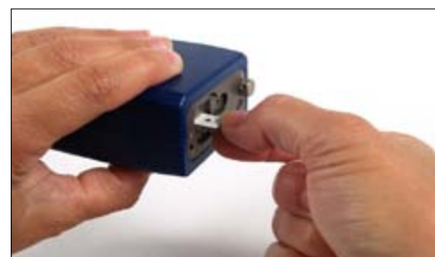
Figure 9: Inserting and removing filter strip while depressing filter release button on bottom of microAeth AE51.
