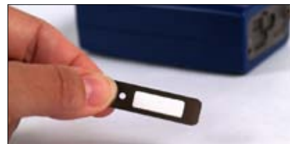
Figure 8: Metal side of filter strip faces the bottom.
