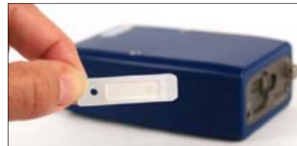
Figure 7: White sample deposit side of filter strip faces the top.
